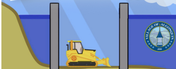
COFFERDAMS CREATE DRY CONSTRUCTION WORK AREAS
