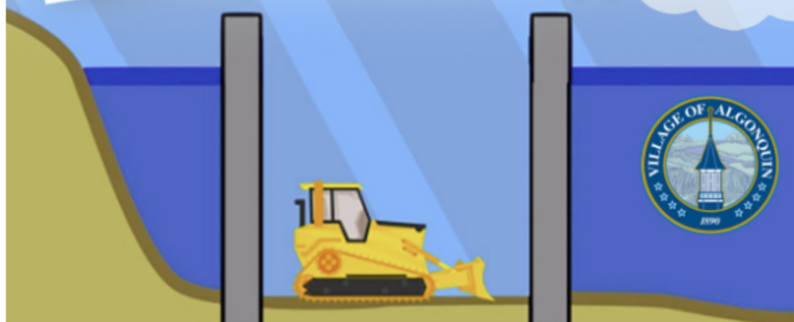
COFFERDAMS CREATE DRY CONSTRUCTION WORK AREAS
