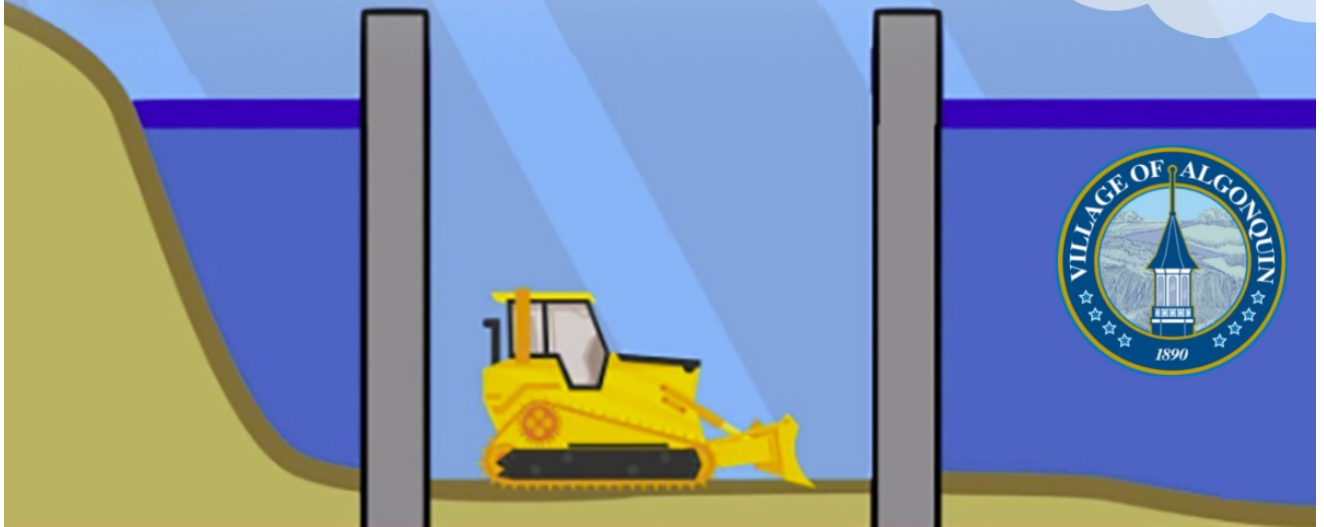
COFFERDAMS CREATE DRY CONSTRUCTION WORK AREAS
